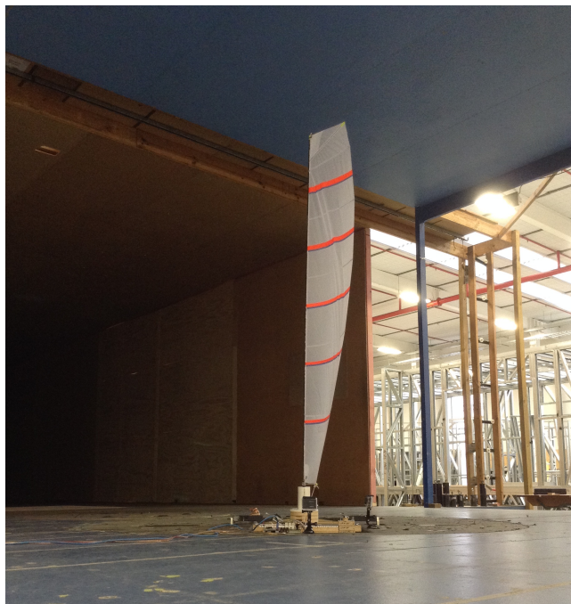
Figure 1. Model mainsail in YRU Twisted Flow Wind Tunnel, University of Auckland
