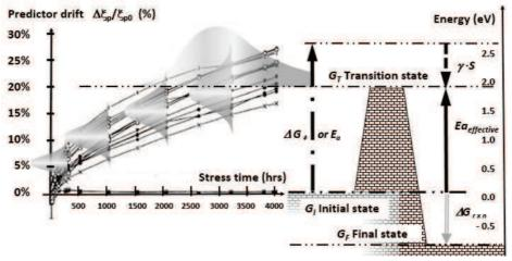
Figure 4: Predictor  $\xi_p$  and Stressor S for BAZ model and Transition State Theory
