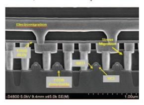
Figure 5. Wear-out phenomena localization (65 nm IC cross section) (from [61]).
