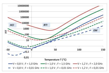
Figure 6: Reliability curves for 45nm technology showing FIT versus Temperature for Voltages above and below nominal (1.2V) and frequencies from 10 MHz (dashed line) to 2GHz (solid line).
