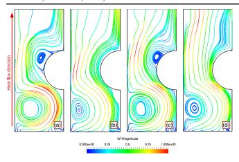
FIG. 3. Streamlines of the normal fluid component. (a)  $T_b=2.0~\rm K,~\dot{q}=25~\rm kW/m^2,~\gamma=620,~a=0.68;$  (b)  $T_b=1.8~\rm K,~\dot{q}=25~\rm kW/m^2,~\gamma=300,~a=1.88;$  (c)  $T_b=1.9~\rm K,~\dot{q}=37\rm kW/m^2,~\gamma=633,~a=0.97;$  (d)  $T_b=1.6~\rm K,~\dot{q}=25~\rm kW/m^2,~\gamma=288,~a=3.1.$
