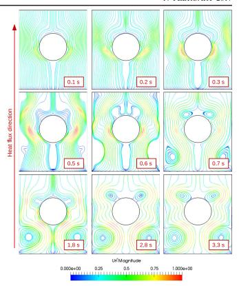
FIG. 2. Streamlines of the normal fluid component past a cylinder at early time steps.
