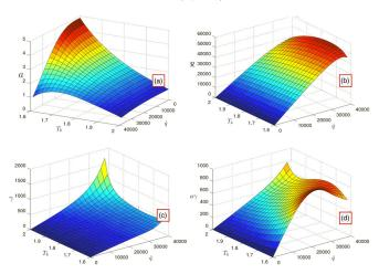
FIG. 1. Variation of the dimensionless numbers with heat flux and bath temperature, (a) densities ratio a, (b) Reynolds number  $\Re$ , (c) mutual friction over the advection of the normal component  $\gamma$ , and (d) mutual friction over the advection of the superfluid component  $a\gamma$ .
