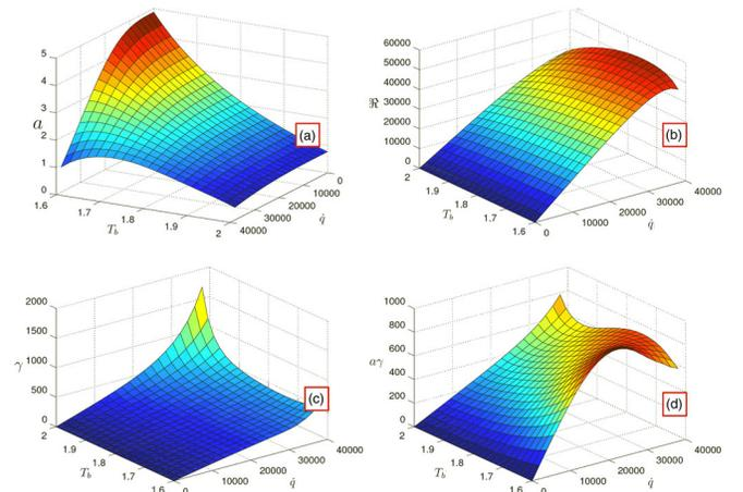
FIG. 1. Variation of the dimensionless numbers with heat flux and bath temperature, (a) densities ratio  $a$ , (b) Reynolds number  $\Re$ , (c) mutual friction over the advection of the normal component  $\gamma$ , and (d) mutual friction over the advection of the superfluid component  $a\gamma$ .
