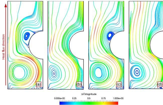
FIG. 3. Streamlines of the normal fluid component. (a)  $T_b = 2.0$  K,  $\dot{q} = 25$  kW/m<sup>2</sup>,  $\gamma = 620$ ,  $a = 0.68$ ; (b)  $T_b = 1.8$  K,  $\dot{q} = 25$  kW/m<sup>2</sup>,  $\gamma = 300$ ,  $a = 1.88$ ; (c)  $T_b = 1.9$  K,  $\dot{q} = 37$  kW/m<sup>2</sup>,  $\gamma = 633$ ,  $a = 0.97$ ; (d)  $T_b = 1.6$  K,  $\dot{q} = 25$  kW/m<sup>2</sup>,  $\gamma = 288$ ,  $a = 3.1$ .
