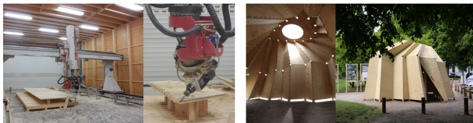
Fig. 8. Digital device of manufacturing and Assembled structure.
