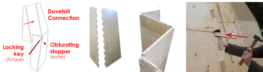
Fig. 9. Woodworking joints
