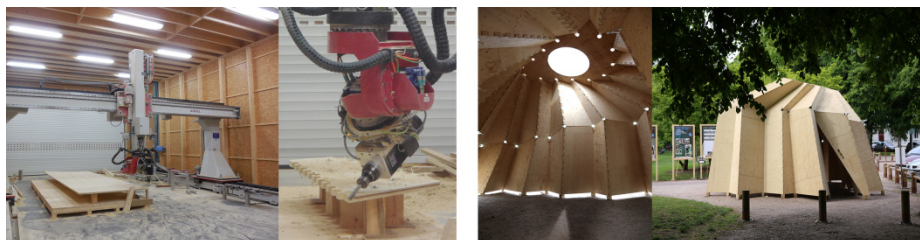
Fig. 8. Digital device of manufacturing and Assembled structure.
