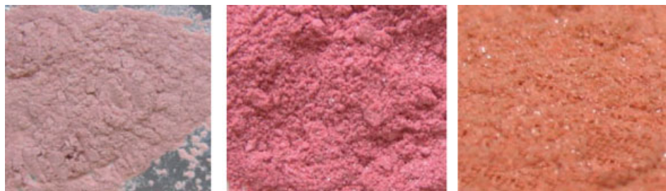
■ Figure 9. Photographs of P(S-A)-mica hybrids for 1, 2, and 4 hours of polymerization, from left to right.
