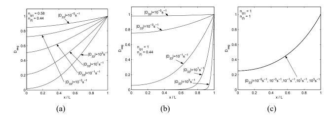
**Figure 2.** Influence of the strain rate  $D_{33}$  on the fiber segregation rate  $D_{seg}$  for various pairs  $n_{(p)}$  and  $n_{(f)}$ , L = 100 mm.
