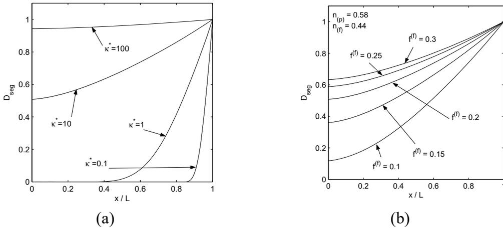
**Figure 3.** Influence of the permeability parameter  $\kappa^*$  (a) and the fiber volume fraction  $f^{(f)}$  (b) on the segregation rate  $D_{seg}$ .
