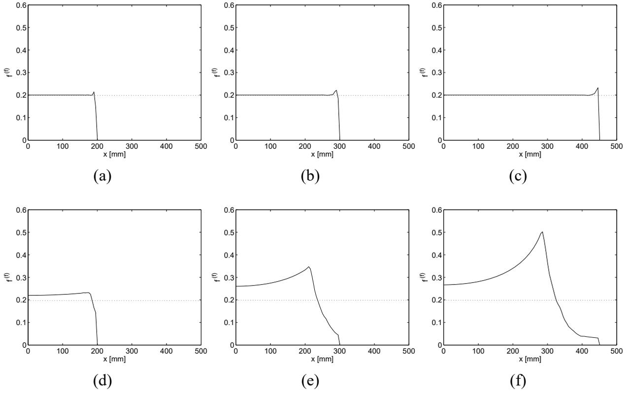
**Figure 4.** Fiber volume fraction profiles during the channel compression tests at various filling times and for two values of the matrix viscosities:  $\mu_{0(m)} = 55000 \text{ Pa s}$  (a-c) and  $\mu_{0(m)} = 550 \text{ Pa s}$  (d-f).
