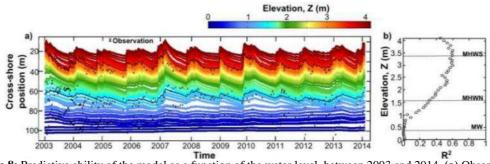
**Figure 8:** Predictive ability of the model as a function of the water level, between 2003 and 2014. (a) Observed (crosses) and simulated (colored lines) cross-shore contour position equilibrium model as a function of the water level (b) R<sup>2</sup> value for contour ranging from 0 to 4.1 m.
