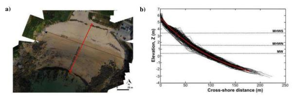
**Figure 2: a)** Planview of the morphological characteristics of the Porsmilin beach. **b)** Cross-shore profiles at Porsmilin from January 2003 to January 2014, indicating mean beach profile (red profile) and Mean High Water Spring (MHWS) level, Mean High Water Neap (MHWN) level and Mean Water (MW) level.
