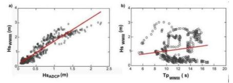
Figure 4: a) Scatter diagram of the significant wave height modèle WWIII (H<sub>swwIII</sub>) and significant wave height ADCP (Hs<sub>ADCP</sub>) and peaks period WWIII (Tp<sub>wwIII</sub>), the solid red line is the regression linear giving y = 1.5920x+0.1548. b) Scatter diagram of the significant wave height model WWIII (HswwIII) and peak period model WWIII (TpwwIII), the solid red line is the regression linear giving y=0.5593x-3.6545.
