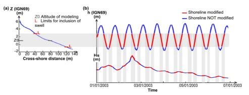
**Figure 5:** Diagram showing how the water level is taken into account in the equilibrium model **(a)** beach profile with the selected elevation contour Z0 and modeling threshold L, **(b)** tide level determining the times periods (red) when the wave forcing the cross-shore position.
