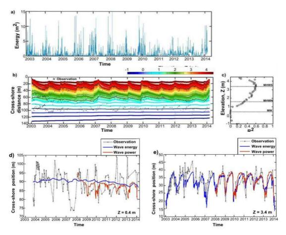
Figure 6: Wave conditions, predictive ability of the model, and R2 values for ranging from -1 to 4.4 m for wave energy (m<sup>2</sup>) (2003-2014) (a), (b), and (c). The predictive ability of the model in (b) compares the observed (crosses) and equilibrium model simulation (colored lines) cross-shore contour positions. Cross-shore observation and the model simulation when the model is forced with the wave energy and wave power. (d) Elevation 0.4 m. (e) Elevation 3.4 m.
