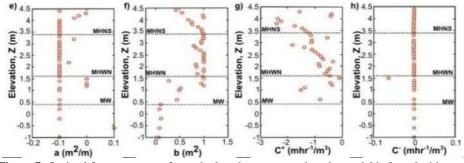
**Figure 7:** Optimal free parameters for each elevation contour when the model is forced with wave energy (**a**, **b**) and wave power (**e**,**h**): (**a**,**e**) Equilibrium slope a, (**b**, **f**) Equilibrium wave energy intercept b, (**c**,**g**) accretion coefficient C<sup>+</sup>, and (**d**, **h**) erosion coefficient C<sup>-</sup>.
