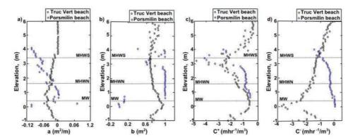
**Figure 11:** Optimal free parameters on the Truc Vert beach (Castelle et *al.* 2014) and Porsmilin beach: (a) equilibrium slope a,. (b) intercept the equilibrium wave energy b,. (c) accretion coefficient C<sup>+</sup>, and (d) erosion coefficient C<sup>-</sup>.
