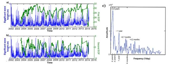
Figure 3: Empirical Orthogonal Functions (EOF) analyses from 2002 to 2014. (a) Correlation between significant wave height (Hs) and the (a) first EOF and (b) second EOF. (c) Spectral analysis of temporary amplitude.
