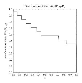
**Fig. 12** The  $|R_t|/\mu R_n$  distribution of the quasistatically deformed block
