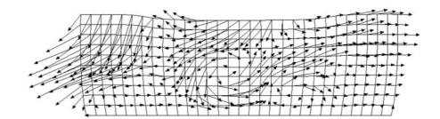
**Fig. 16** The nodes velocity field at  $0.2 \times 10^{-3}$  s after the projectile has bounced off the block
