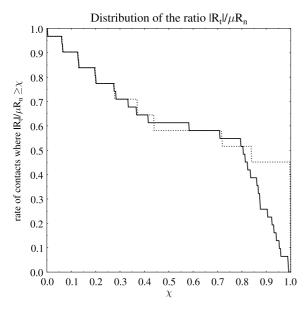
Fig. 15 The  $|R_t|/\mu R_n$  distribution of the settled impacted block
