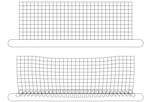
**Fig. 11** The quasistatically deformed block at equilibrium and the reaction forces at the nodes
