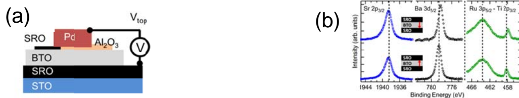
Figure 1: (a) Schematic of the SRO/BTO/SRO heterostructure, (b) Hard x-ray photoemission spectra for both polarization states in a SRO/BTO/SRO capacitor measured at 6.9 keV. The binding energy shift in the core-level of the FE layer (Ba 3d 5/2 and Ti 2p 3/2 here) is due to the different interface potential when switching polarization.
