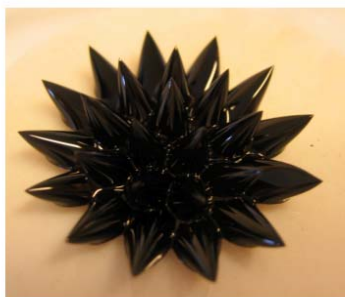
Figure. Left panel: Magnetic instability of ferrofluids; Right panel: \text{CoFe}_2\text{O}_4 nanospinels present in ferrofluids (scale bar 10nm).
