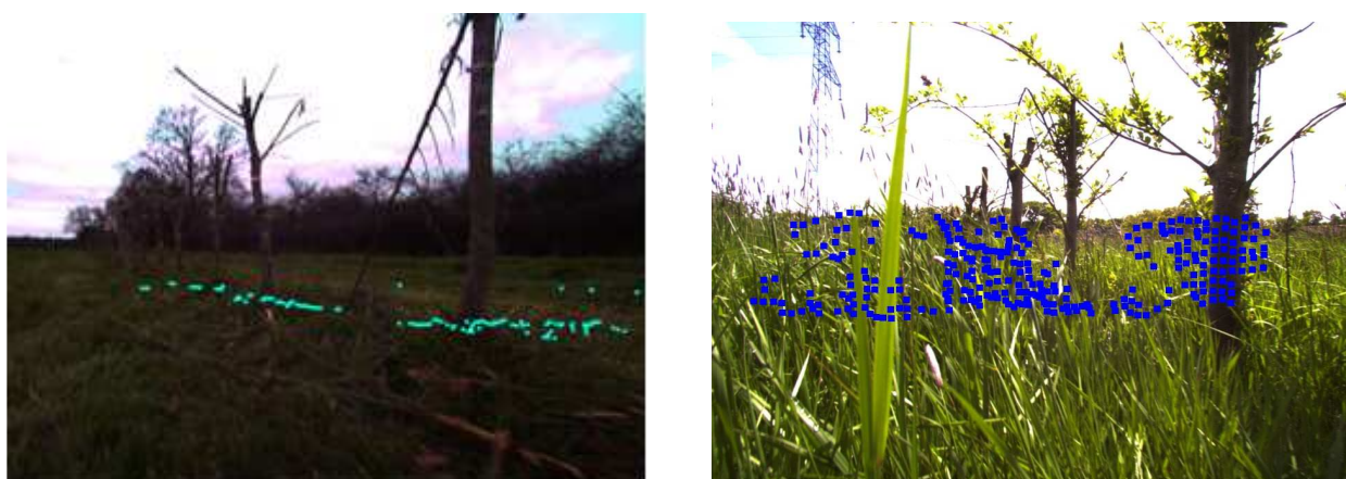
(a) (b) Figure 4. Positioning of lidar (a) and TOF (b) data on color images
