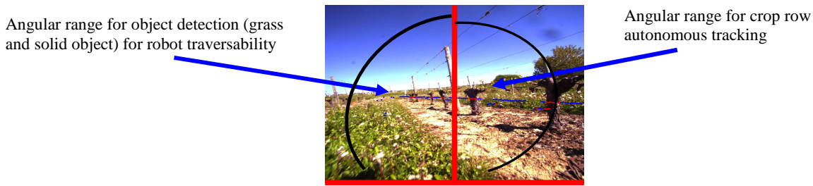
Figure 12. Lidar data areas for crop raw tracking (tree detection) and object identification for traversability
