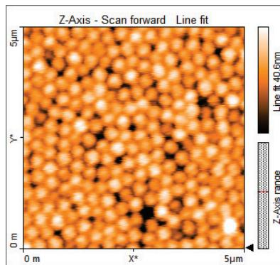
**Figure 3:** Zoom of an AFM height scan of a monolayer of dried core-shell microgels with 5 mol% core crosslinker content. The lateral image size is 5  $\mu\text{m}$  and the average height is 30.8 nm.
