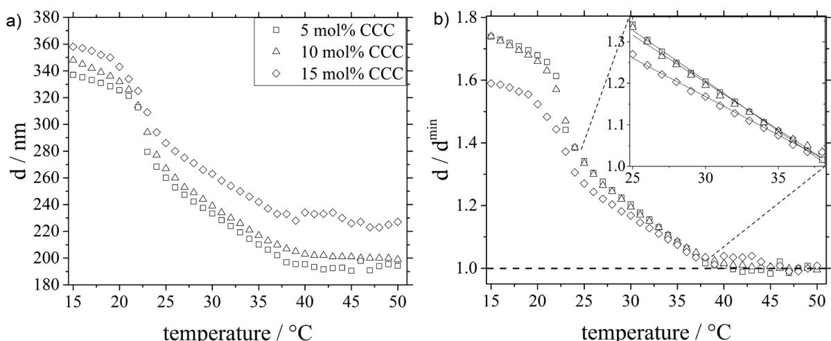
**Figure 4:** Ellipsometric measurements in water of the **a)** layer thickness  $d$  of core-shell microgels deposited on a silicon wafer, for different core crosslinker contents as indicated in the legend, as a function of temperature. In **b**,
