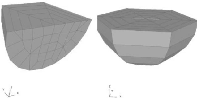
Fig. 17. Samples of lower plenum meshings (CFD solver).
