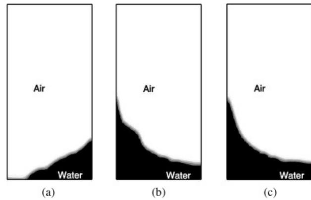
Fig. 3. Maschek test case: computational maxima of the calculation performed with NEPTUNE CFD on a  $33 \times 45$  cartesian mesh, represented by the water fraction field: (a) first motion toward the wall; (b) first peak; (c) second peak; (2-D axisymmetrical computation).
