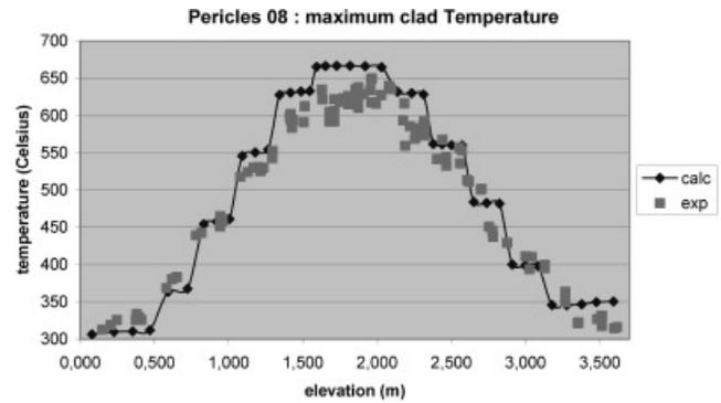
Fig. 14. Maximum clad temperature profile in PERICLES Reflooding Test 8: comparison of experiment with a three-field model prediction.
