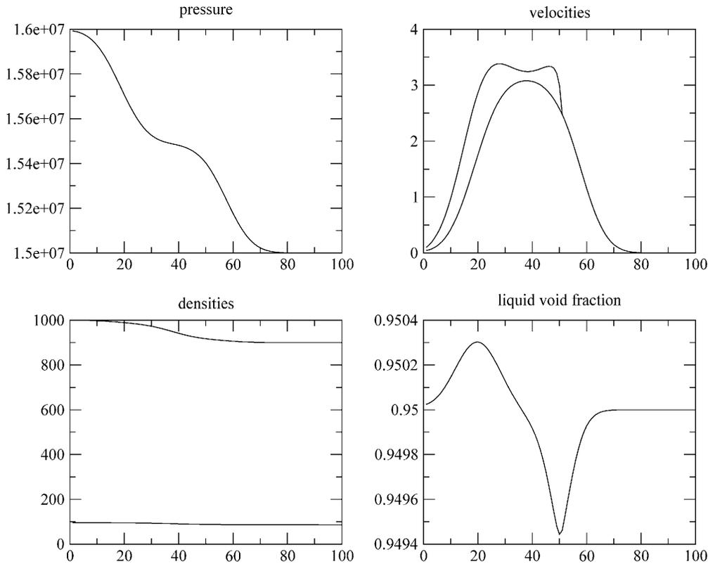
Fig. 22. Propagation of waves through the coupling interface when coupling a two-fluid model (left side) and a homogeneous model (right side).
