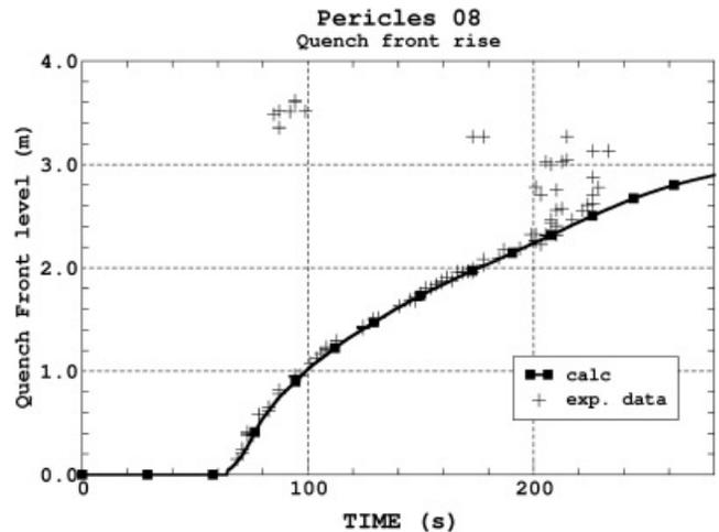
Fig. 15. Quenching time in PERICLES Reflooding Test 8: comparison of experiment with a three-field model prediction.
