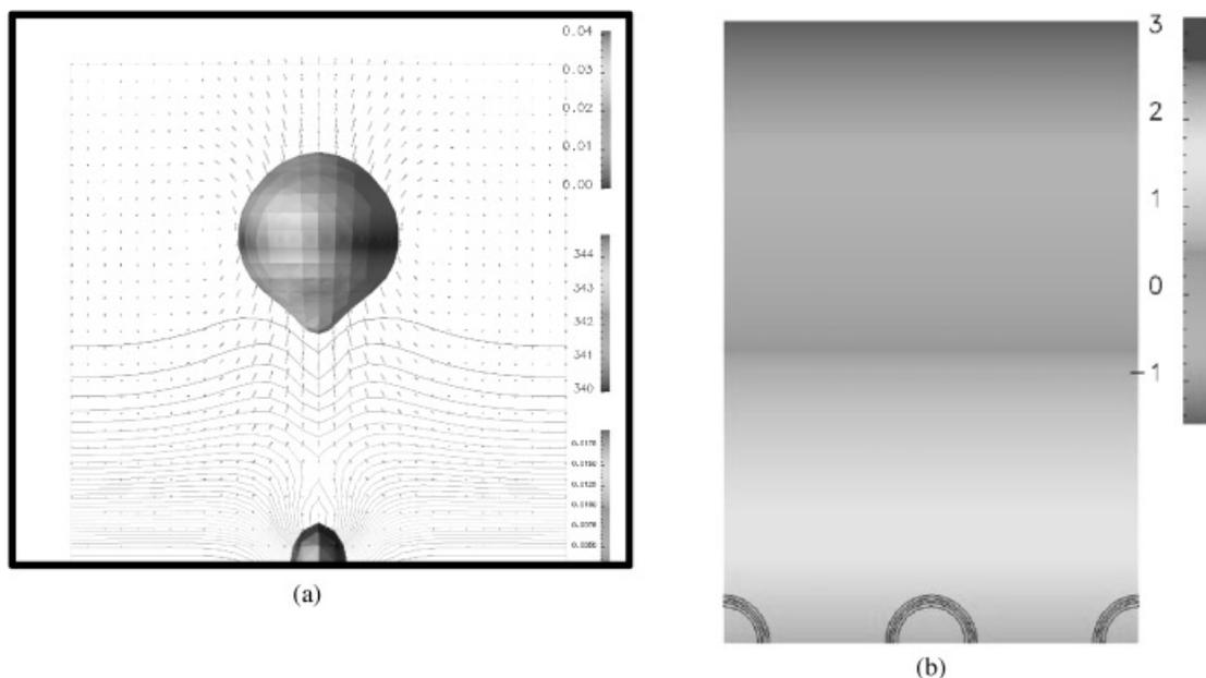
Fig. 23. DNS simulation of (a) monosite boiling by Mathieu et al.,<sup>95</sup> and (b) multisite boiling by Fouillet.<sup>96</sup>
