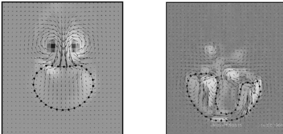
Fig. 25. Simulation with LES coupled to an interface tracking technique. Distortion of a bubble due to large-scale eddies (Labourasse et al.<sup>98</sup>).
