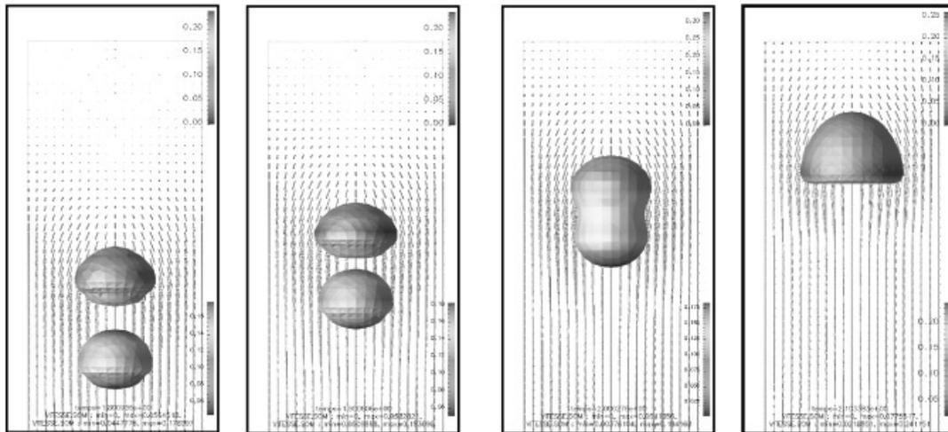
Fig. 24. DNS simulation of a coalescence of two bubbles (Mathieu<sup>97</sup>).
