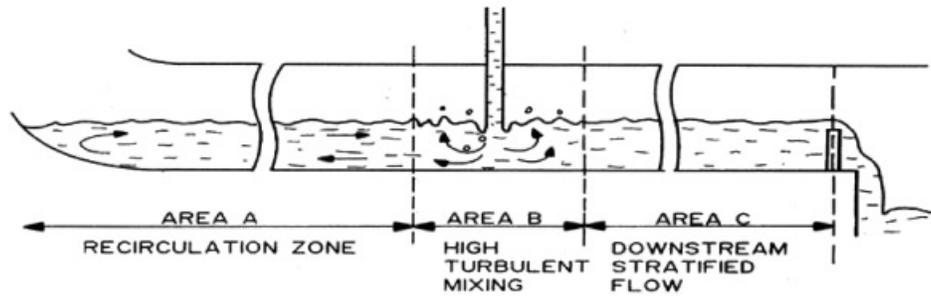
Fig. 7. Flow configuration in COSI tests.
