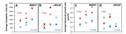
**Fig. 4** For both tests, average incubation times for **a** 800HT and **b** HR120 samples and average lateral pit growth rate constants for a given side of **c** 800HT and **d** HR120 samples. *Full* and *empty symbols* are data obtained on the external and internal side of the samples respectively
