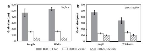
Fig. 1 Alloy grain size measured by image analysis on  $\mathbf{a}$  the surface and  $\mathbf{b}$  the cross-section. For measurements at the surface of the circular samples tested at 21 bar, length and width are two normal directions
