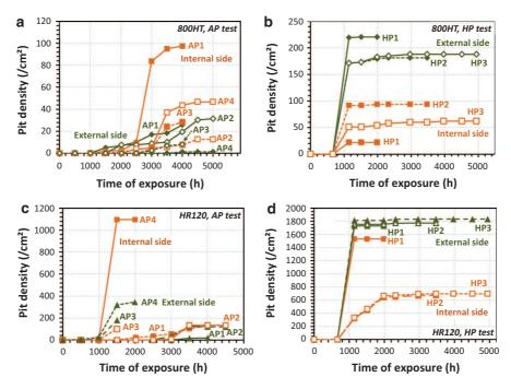
Fig. 3 Pit density versus exposure time for 800HT at **a** 1 bar and **b** 21 bars and for HR120 at **c** 1 bar and **d** 21 bar
