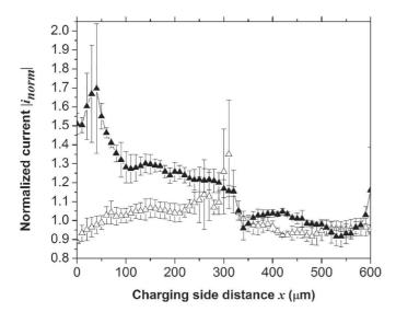
**Fig. 2.** Evolution of the AC-SECM normalized currents after charging for 15 h as a function of the distance *x* from the H-charging side ( $\blacktriangle$ ) and after an additional heat treatment for 2 h at 130 °C ( $\Delta$ ).
