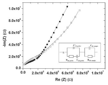
**Fig. 3.** Typical localized impedance spectra obtained in the H-containing zone ( $\blacksquare$ ) and in the H-free zone ( $\square$ ) for a 15 h H-charged AA 2024 sample. Measurements were performed in 1 mM Na<sub>2</sub>SO<sub>4</sub>. Frequency range: 100 kHz–500 Hz. The solid lines show the fitting to the equivalent circuit presented in the insert.
