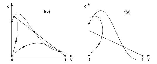
Figure 2. Schematic representation of the phase plane of system (4), (5). There are 6 stationary points in the left figure. Two of them are stable (see the explanation in the text). The function f(v) becomes negative for large v in the right figure. There are also two stable stationary points, the most left and the most right ones.
