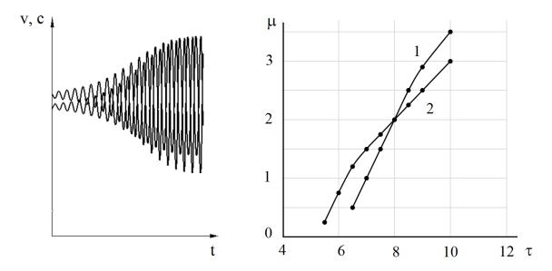
Figure 3. Example of periodic oscillations for the values of parameters  $k = \sigma = 1$ ,  $\phi(v) = 2v$ ,  $\psi(v) = v$ ,  $\tau = 10$ ,  $\mu = 2$  (left). Stability boundary on the  $(\tau, \mu)$  plane for  $k = \sigma = 1$  (right): Curve 1 is defined by  $\phi(v) = 3v$ ,  $\psi(v) = v$ , and curve 2 by  $\phi(v) = 2v$ ,  $\psi(v) = v$ . The stability region is located above the curves.
