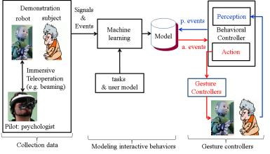
Figure 3. The three main steps of learning interaction by demonstration: collecting HRI data, learning a behavioral model and building appropriate sensorimotor controllers.
