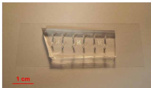
Fig. A1 Picture of the PDMS experimental chip. The PDMS is bonded on a glass cover slip.
