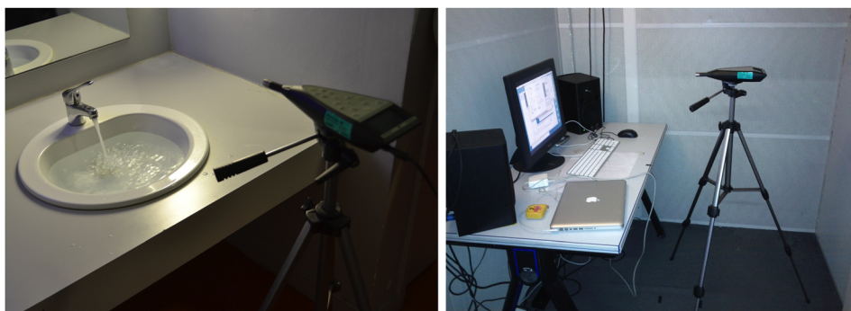
FIG. 2. (Color online) Calibration of a recording sound to obtain the same level (in dBA peak) in the listening cab as under real conditions in a bathroom.
