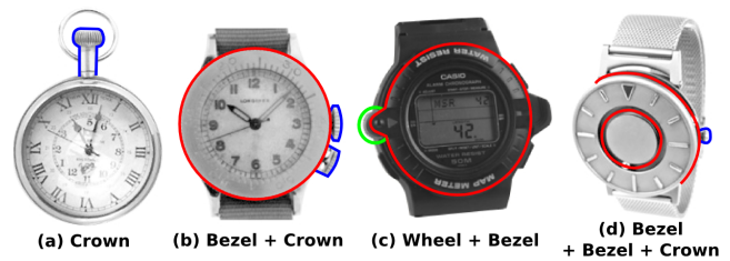
Figure 1: Examples of watch combining different types of rotary inputs
