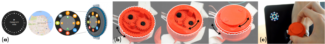
Figure 5: (a) The three implemented applications and the envisioned device. (b) Our proof-of-concept, a watch using two stacked bezels. The bottom bezel is toothed, the top bezel is slanted. (c) For demos, we used a deported screen when visual feedback was necessary
