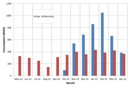
Figure 7 : Total energy consumption from May-2014 to Apr-2015
