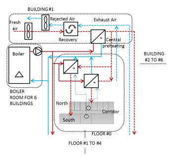
Figure 3. AHU and water systems provide indoor ventilation
