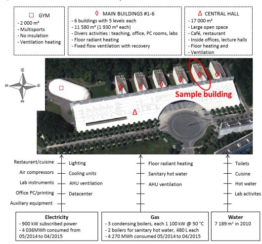
Figure 2. Details of the studied site – buildings, utilities and energy supplies. The red circle indicates the sample considered for instrumentation, measurements and building energy model validation presented in the following sections.
