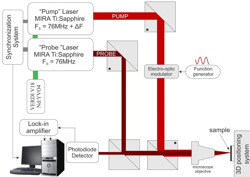
FIG. 2. High-throughput pump-probe thermoreflectance setup.
