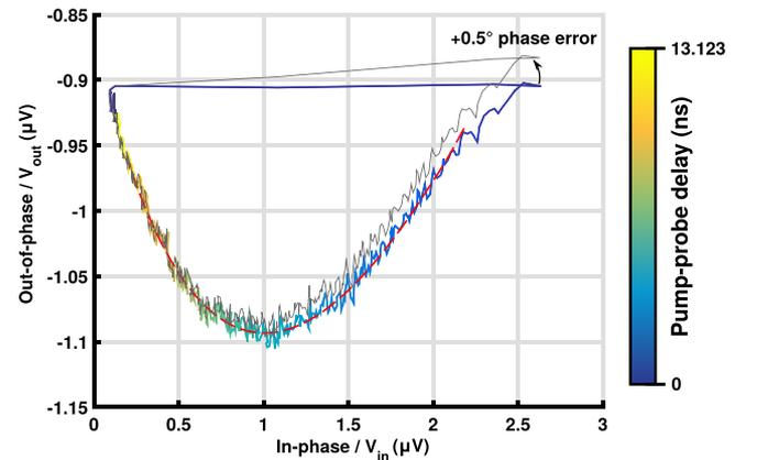
FIG. 4. Nyquist plot  $V_{out}(t) = f(V_{in}(t))$  for  $\text{Fe}_{36}\text{Si}_{28}\text{Ge}_{36}$ . Solid line is the measured lock-in amplifier signal in the Nyquist plane and is colored according to time, from dark blue for a zero pump-probe delay to bright yellow for 13.123 ns. Dashed red line is the best fit obtained. Grey line is the measured lock-in amplifier signal with a +0.5° phase error.
