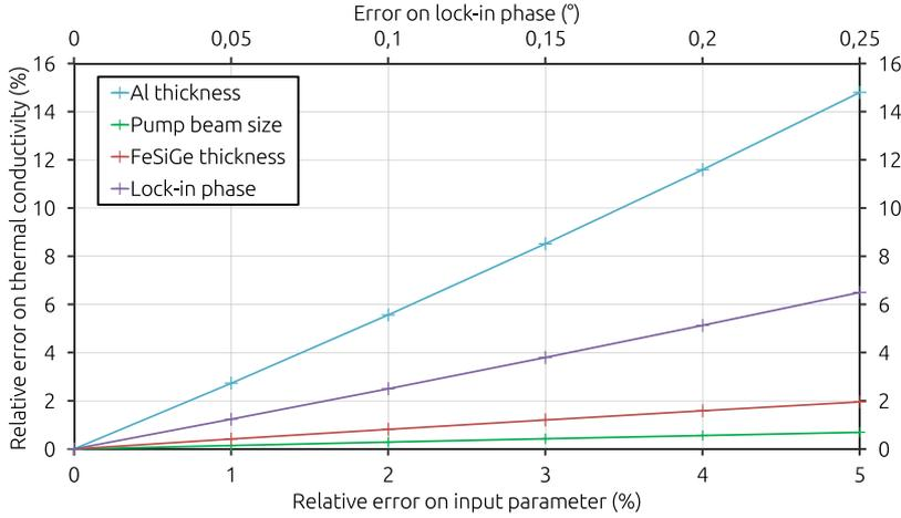
FIG. 3. Plot of the error on the identified thermal conductivity for a relative variation of four different input parameters for  $\text{Fe}_{70}\text{Si}_{29}\text{Ge}_1$ . Blue (respectively, red, green, and purple) lines refer to the input Al thickness (respectively, Fe-Si-Ge thickness, pump beam size, and lock-in phase). Simulated parameter values are as follows: Al thickness: 70 nm; Fe-Si-Ge thickness: 354 nm; pump beam size: 9.5  $\mu\text{m}$ .
