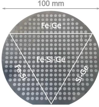
FIG. 1. Ternary Fe-Si-Ge alloy library deposited on a 100 mm sapphire wafer.
