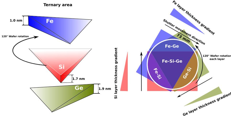
FIG. 5. Schematic of the wedge-type multi-layer deposition method.
