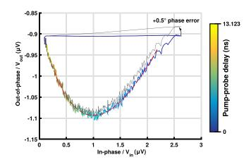
FIG. 4. Nyquist plot  $V_{out}(t) = f(V_{in}(t))$  for  $Fe_{36}Si_{28}Ge_{36}$ . Solid line is the measured lock-in amplifier signal in the Nyquist plane and is colored according to time, from dark blue for a zero pump-probe delay to bright yellow for 13.123 ns. Dashed red line is the best fit obtained. Grey line is the measured lock-in amplifier signal with a  $+0.5^{\circ}$  phase error.
