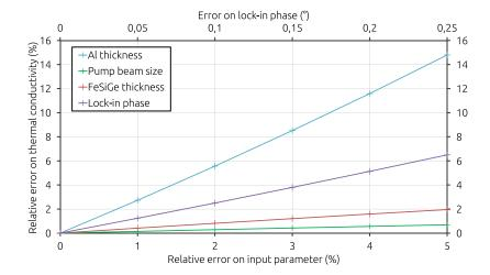
FIG. 3. Plot of the error on the identified thermal conductivity for a relative variation of four different input parameters for Fe $_{70}$ Si $_{29}$ Ge $_1$ . Blue (respectively, red, green, and purple) lines refer to the input Al thickness (respectively, Fe-Si-Ge thickness, pump beam size, and lock-in phase). Simulated parameter values are as follows: Al thickness: 70 nm; Fe-Si-Ge thickness: 354 nm; pump beam size: 9.5  $\mu$ m.
