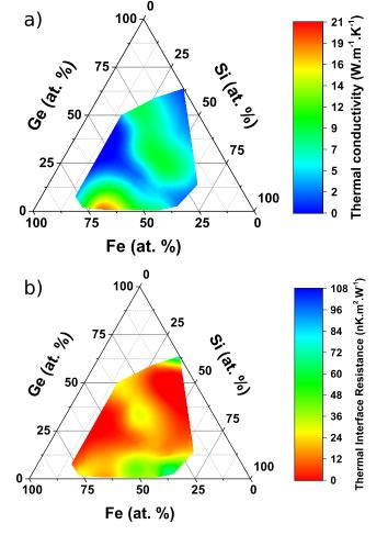
FIG. 7. (a) Ternary graph of measured thermal conductivities on a multiwedge deposited Fe-Si-Ge alloy library. (b) Ternary graph of the measured thermal interface resistances on a multi-wedge deposited Fe-Si-Ge alloy library.
