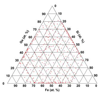
FIG. 6. Compositions in the Fe-Si-Ge thin film library as determined by high-throughput EDX measurements.
