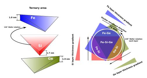
FIG. 5. Schematic of the wedge-type multi-layer deposition method.
