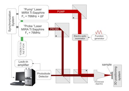
FIG. 2. High-throughput pump-probe thermoreflectance setup.
