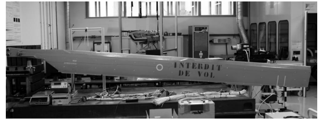
Fig. 10 Helicopter blade used as primary structure.
