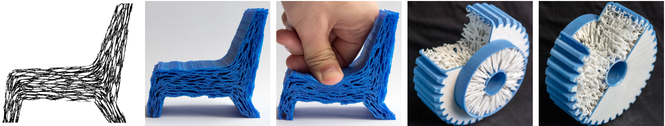
Fig. 1. 3D printed objects. Left: A comfy chair inspired by the work of designer Lilian van Daal. The orthotropic material is oriented to give a soft response on the seat and the back, while keeping other directions rigid. Right: Illustrative example of a gear made lighter by filling it with an orthotropic microstructure oriented against the surface to resist pressure.
