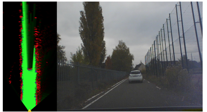
Figure 1: Example of an occupancy grid with its corresponding scene. The yellow triangle represents the position of the Lidar sensor, the green color in the occupancy grid shows the free space, the red shows the occupied space, while the blue represents conflicting cells (before normalization) and the black represents unexplored cells. The color intensity reflects the certainty degree.
