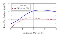
Fig. 2. No-load peak flux-linkage with and without PM
