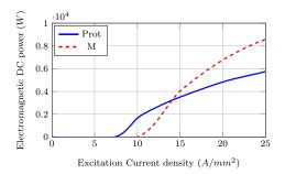
Fig. 20. Electromagnetic DC power comparison at 6000 rpm
