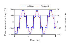
Fig. 9. Phase voltage and phase current for  $I_{exc} = 5 \text{ A}$  at 6000 rpm
