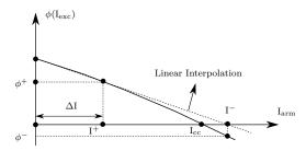
Fig. 13. Short-circuit current calculation using the SFE model
