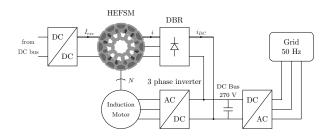
Fig. 10. Scheme of the experimental setup
