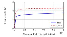
Fig. 5. B-H magnetization curves for CoFe and SiFe
