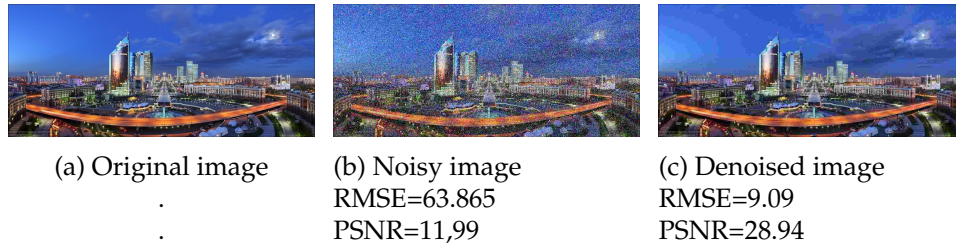
Figure 4.1: From left to right, original image, noisy image corrupted with Salt and Pepper noise with parameter \sigma = 30 and filtered image by proposed algorithm.
