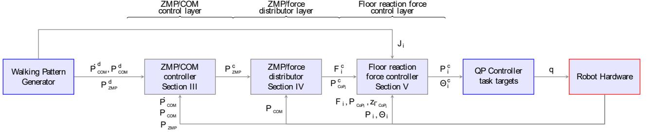
Fig. 2: Overview of the control loop. Superscripts  $d$  and  $c$  denote desired and control references, respectively, while robot measurements have none.  $i \in \{R, L\}$  stands for right or left foot.  $\mathbf{P}$  refers to positions,  $\mathbf{F}$  to forces and  $\Theta$  to orientations.
