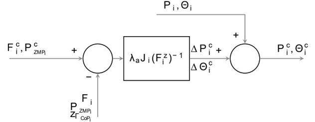
Fig. 6: Reaction force controller: the ZMP  $\mathbf{P}_{ZMP_i}^c$  and contact force  $\mathbf{F}_i^c$  under the foot  $i$  are compared to the robot state  $\mathbf{P}_{ZMP}^c$  and  $\mathbf{F}_i^c$  in order to control in admittance the robot by generating foot  $i$  relative position  $\mathbf{P}_i^c$  and orientation  $\Theta_i^c$  control.
