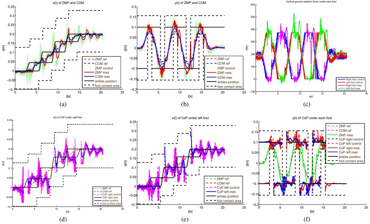
Fig. 8: Walking over gravel (granulometry: 10/20 mm): (a,b) ZMP and COM, (c) Vertical ground reaction forces and (d,e,f) CoP under each foot: measured compared with the references along  $x/y$  axes during a four steps and 20cm long.
