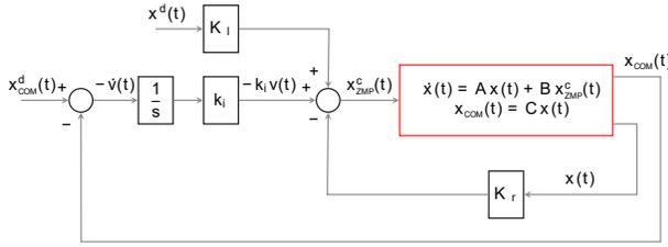
Fig. 3: *ZMP-COM tracking controller*: the state reference  $x^d$  of COM velocity, COM and ZMP position is compared to the measured state  $x$  in order to control the system (in red) with a ZMP control  $x_{ZMP}^c$ .
