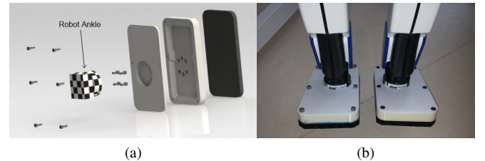
Fig. 7: (a): new HRP-4's feet; (b): photo of HRP-4's feet with soft soles
