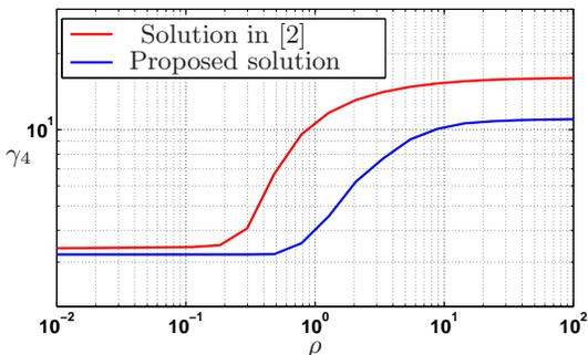
Fig. 2. Upper bounds of the nonlinear  $\mathcal{L}_4$ -gain for the system studied in [2, Example 5.2] obtained by solving inequalities (13) (blue line) and obtained with the coordinate-wise search to solve the BMIs in [2] (red line).
