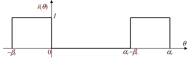
Fig. 3. Power current profile in the phase versus rotor angle
