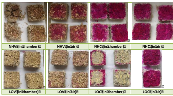
Fig. 15 : 50mm cubes samples after phenolphthalein spray at 6 weeks of curing
