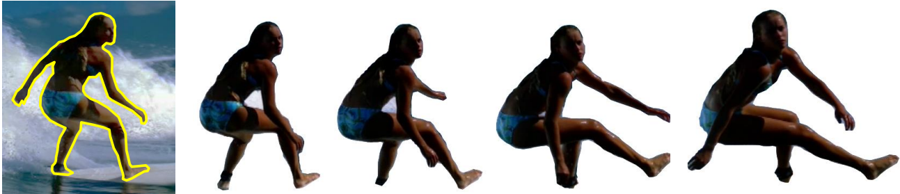
Figure 1: ROAM for video object segmentation. Designed to help rotoscoping , the proposed object appearance model allows the automatic delineation of a complex object in a shot, starting from an initial outline provided by the user.
