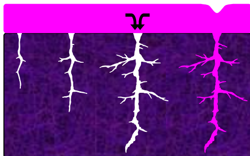
FIG. 9. Spontaneous opening and growth of the internal rip in the condensed matter. The open rip is filled with an alternative material.
