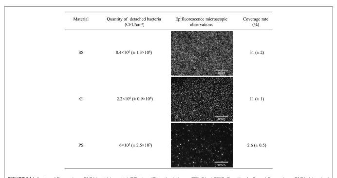
**FIGURE 2** | Adhesion of *P. aeruginosa* PAO1 to stainless steel (SS), glass (G), and polystyrene (PS), 3 h at  $37^{\circ}\text{C}$ . Quantity of adherent *P. aeruginosa* PAO1 determined by enumeration and epifluorescence microscopic observations with a  $\times 20$  objective after SYTO9 staining.
