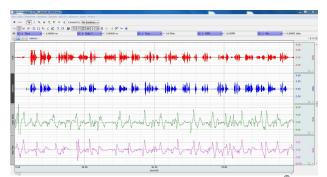
Figure 4: Acquisition of the 4 signals with the  $BIOPAC^{\otimes}$  system. Channel 1 is the children voice recorded by the headset microphone, channel 2 is the master voice output by the tablet delivered via the headphones, channels 3 & 4 are the monitored abdominal vs. thoracic breathing signals.
