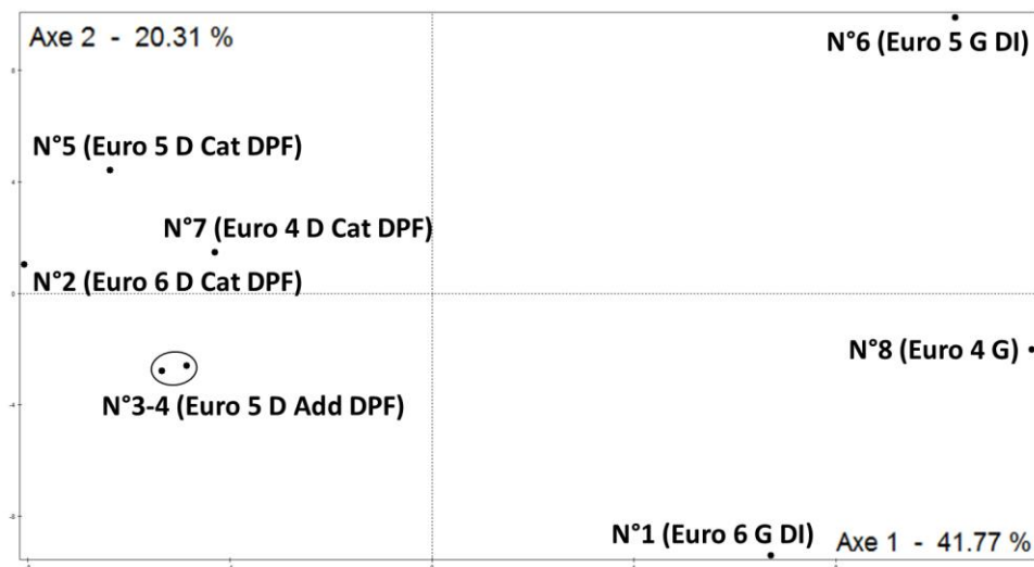
374 Figure 6. PCA performed for all the driving cycles and all the vehicles, with (a) the projection of 375 emission factors and (b) the projection of vehicles.
