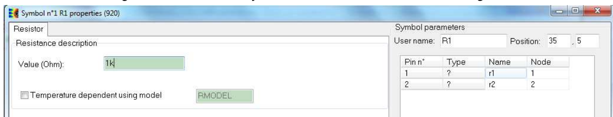
Figure 2- 10: Change the resistance value of a resistor symbol
