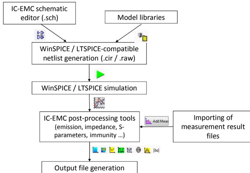
Figure 2- 3: General simulation flow with IC-EMC
