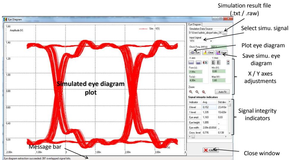
Figure 4- 47: Eye diagram plot (basic\signal\_integrity\ Eye\_digital\_IO\_switching.sch)
