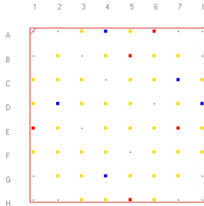
Figure 3- 77: 2D floorplan of a BGA 64 package (examples\ibis\BGA64.ibs)
