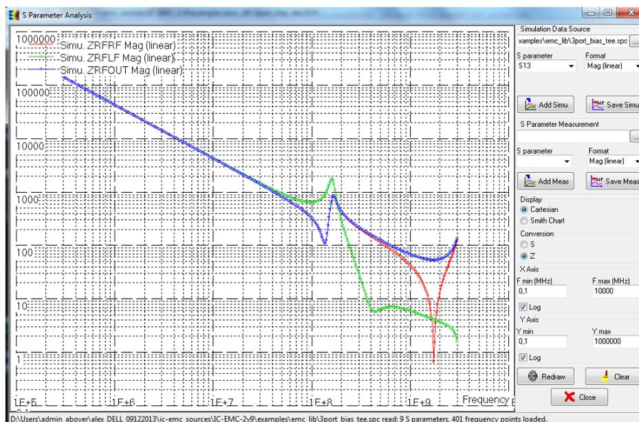
Figure 3- 23: Conversion from S to Z parameters (examples\EMC\_lib\3\_port\_bias\_tee.sch)
