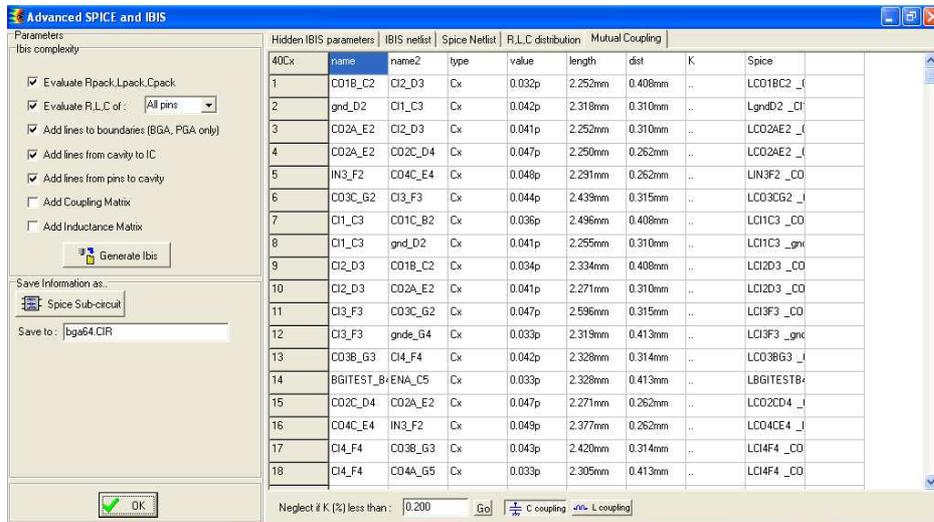
Figure 3- 85: Capacitance coupling listed in IC-EMC (examples\ibis\BGA64.ibs)
