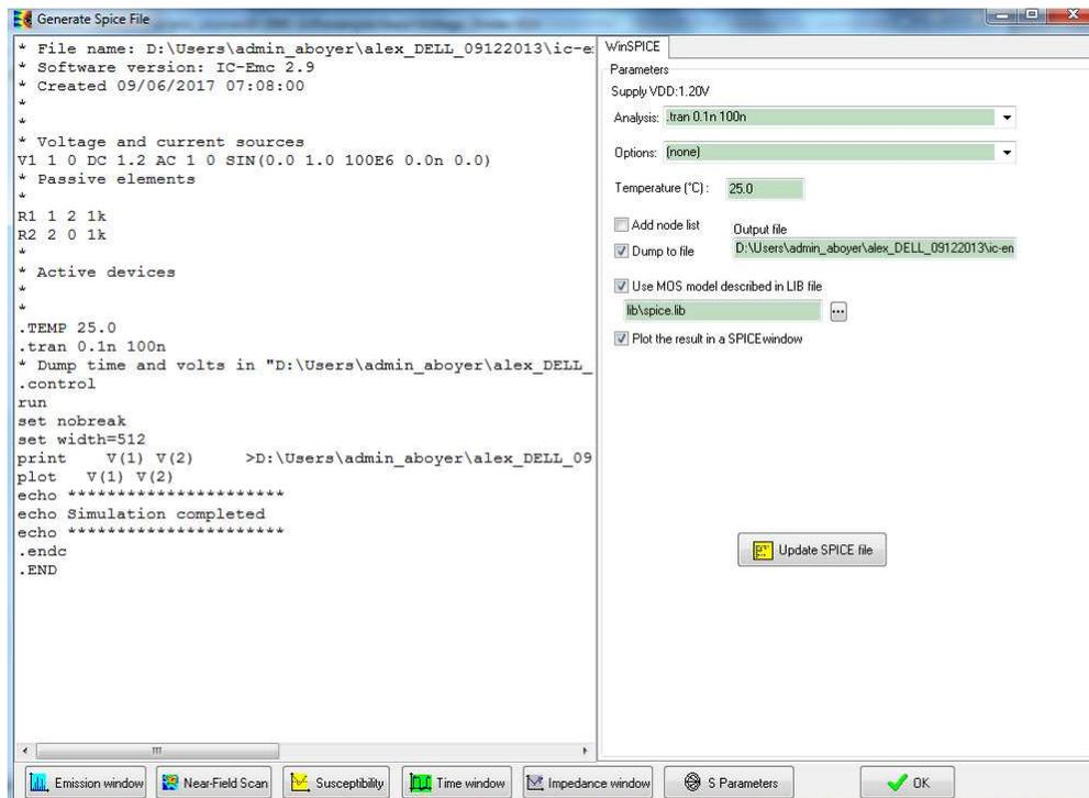
Figure 2- 18: Generation of the netlist file
