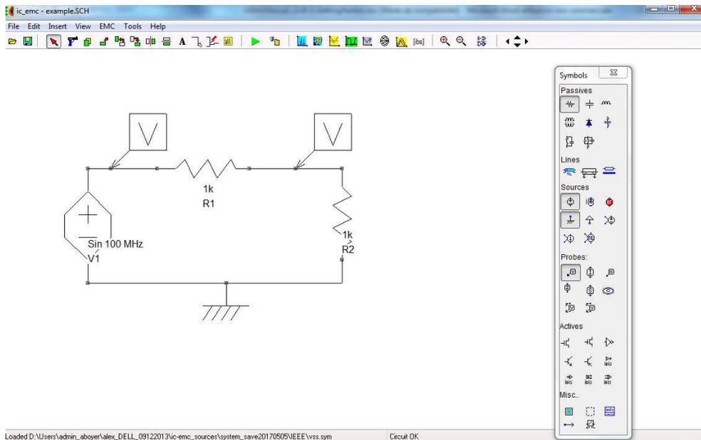
Figure 2- 14: Place voltage probes and the ground symbol
