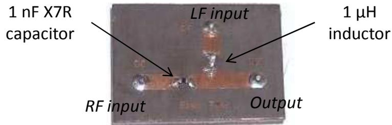
Figure 3- 18: Home-made bias tee for DPI tests
