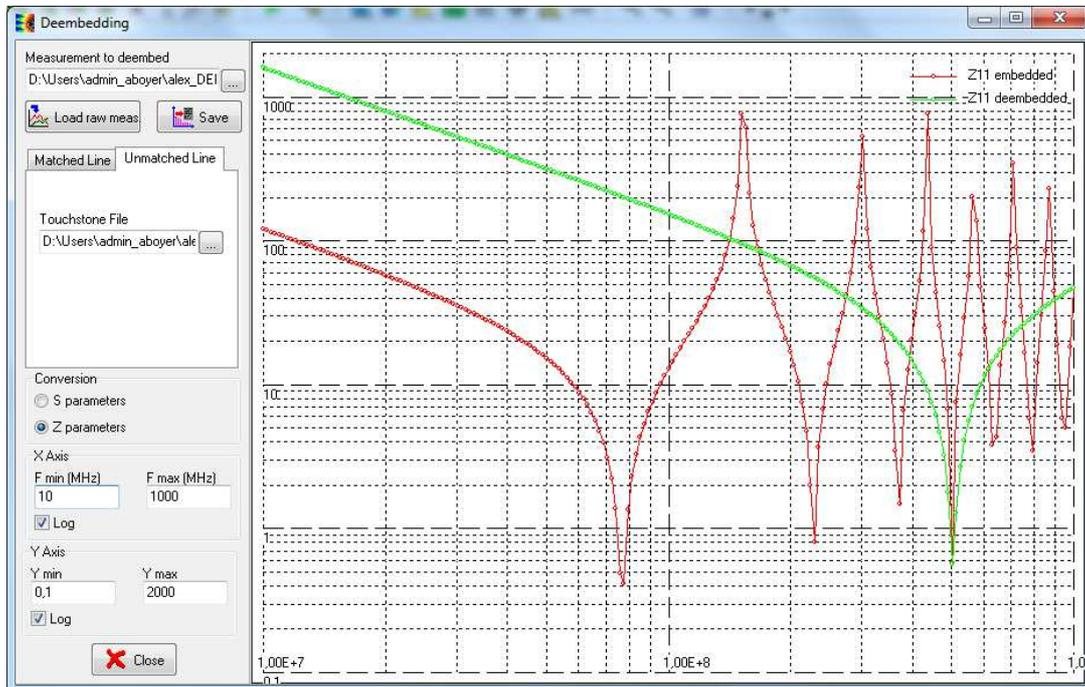
Figure 4- 44: S parameter deembedding user’s interface (examples\basic\deembed\S11\_rawDeembed.s1p)
