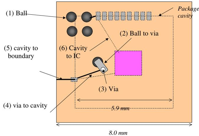
Figure 3- 79: The 6 electrical elements forming each pin of the BGA package
