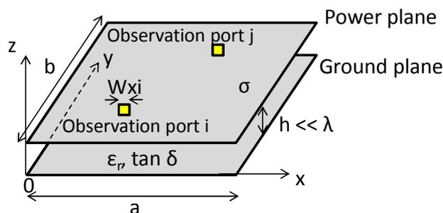
Figure 3- 100 : Rectangular 2D cavity formed by a PG plane pair
