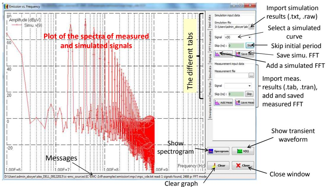
Figure 4- 20: the window "Emission vs. Frequency"
