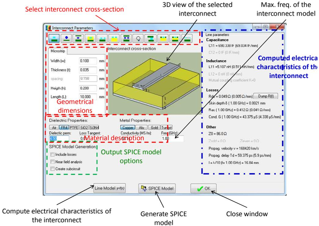
Figure 4- 39: Interconnect R,L,C model based on physical dimensions
