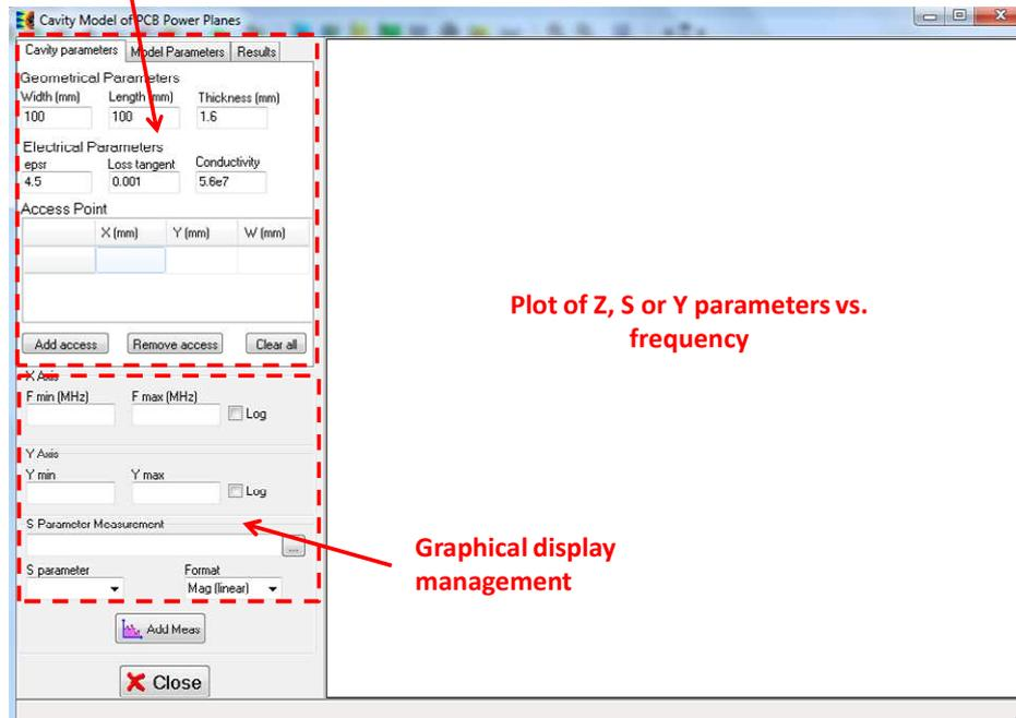
Figure 4- 41: Configuration of cavity dimensions and port placement
