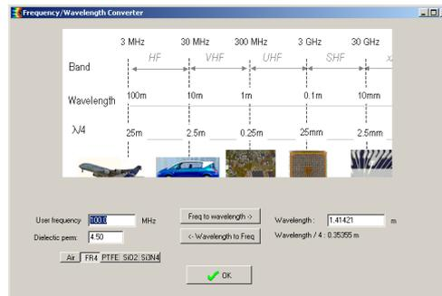
Figure 4- 50: The user's interface for the frequency/wavelength conversion
