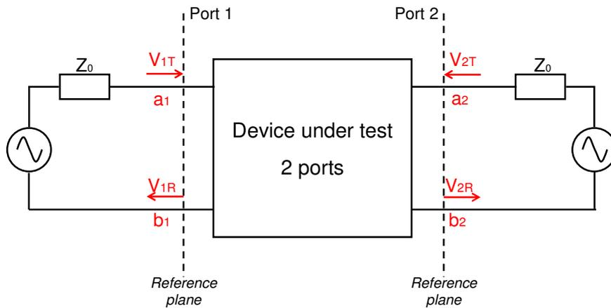
Figure 3- 21 : S parameter characterization of a 2 port device
