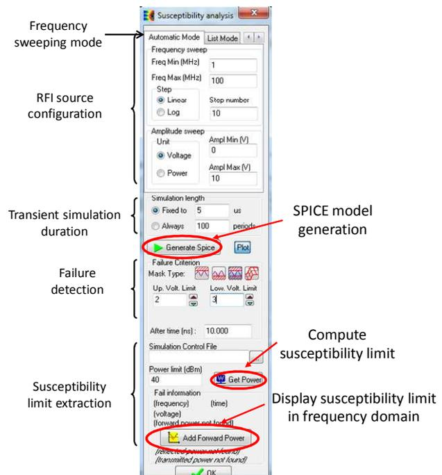
Figure 3- 26: Configuration of the simulation of susceptibility
