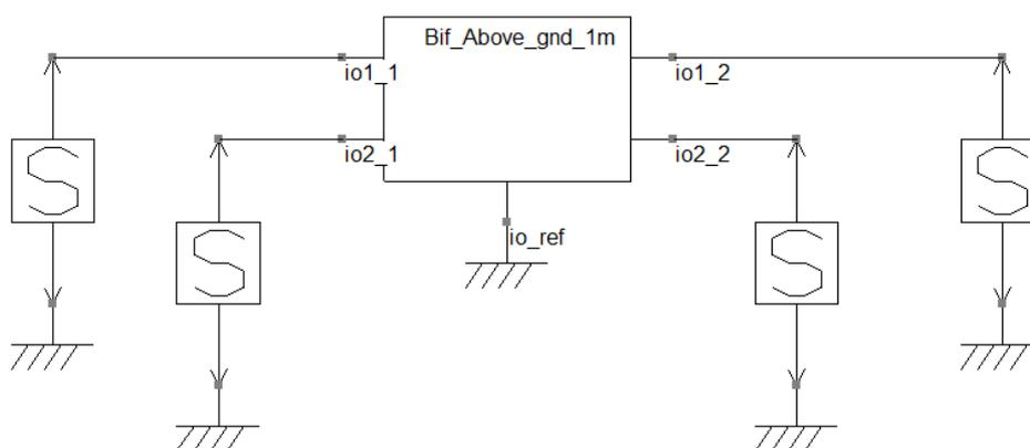
Figure 3- 74: S parameter simulation of a bifilar pair cable
