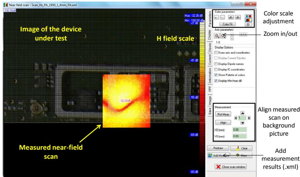
Figure 3- 52: Example of near-field scan with IC-EMC (`\\case_study\pa_3G\Scan_Hx_PA_1950_1_5mm\Scan_Hz_PA_1950_1_8mm_PA.xml`)
