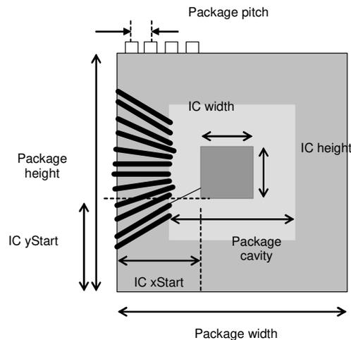
Figure 4- 18: Top view of the package
