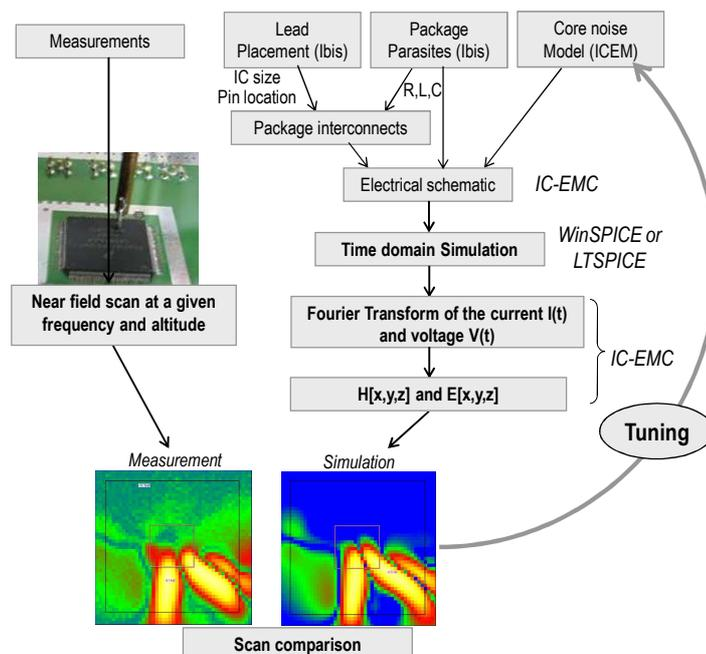
Figure 3- 54: Flow for comparing predicted and simulated magnetic field scans
