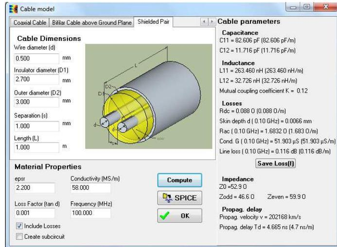
Figure 4- 40: The attenuation in cable evaluation interface
