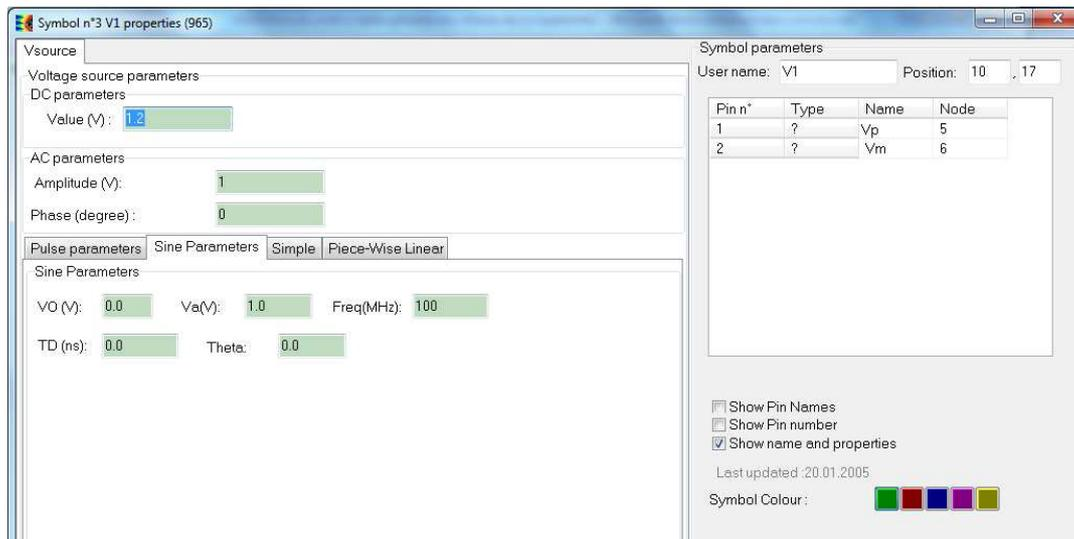
Figure 2- 12: Edit the properties of a voltage source
