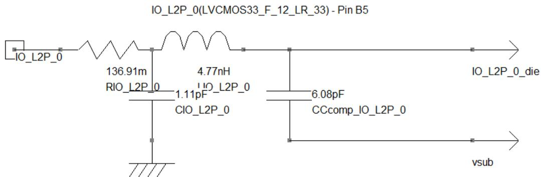
Figure 3- 31: Model of the PT0 pad (examples\libis\ Xilinx\_Spartan6\_LVCMOS33.ibs)
