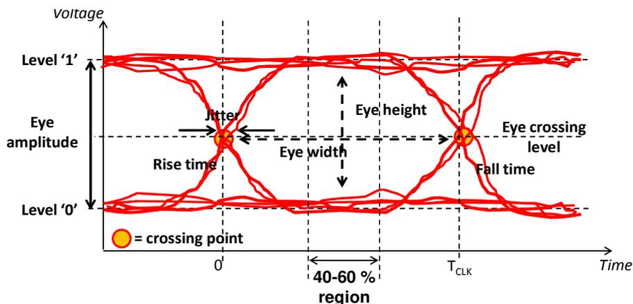
Figure 3- 43: Signal integrity indicators extracted from eye diagram
