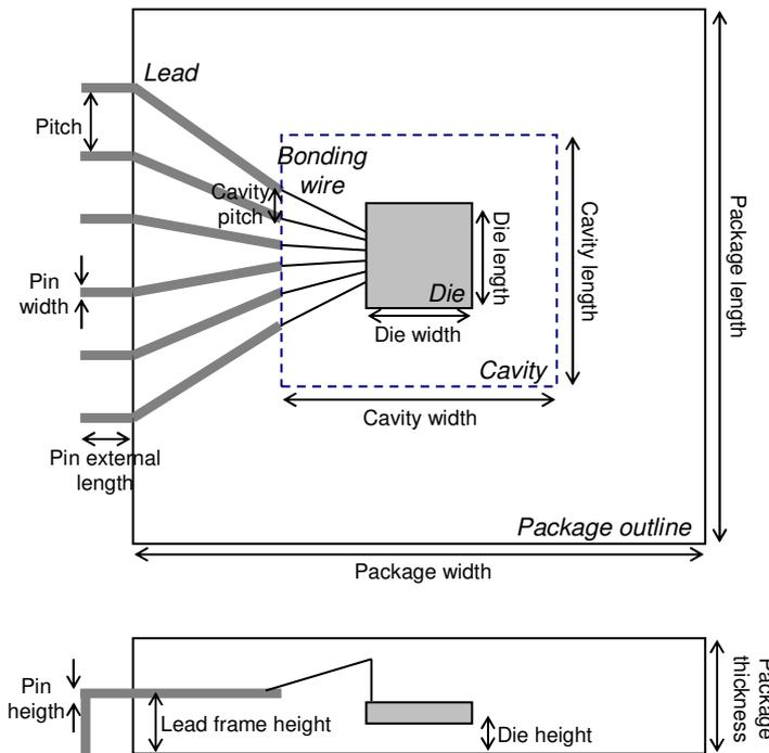
Figure 3- 90 : Interface to define realistic package
