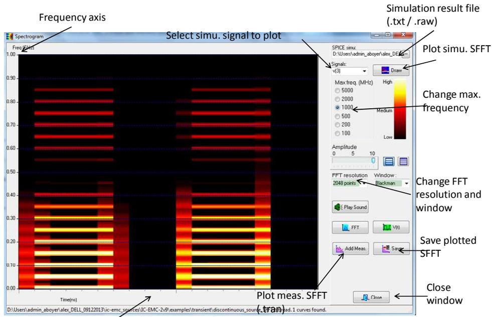
Figure 4- 46: Spectrogram user's interface (examples\transient\ discontinuous\_source\_SFFT.sch)
