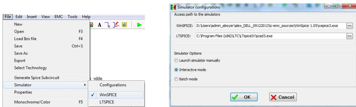
Figure 3- 14: Select simulator and configure the simulator options
