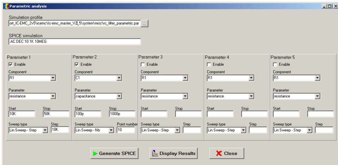
Figure 4- 29: Parametric analysis configuration interface (examples/misc/rc\_filter\_parametric.sch and examples/misc/rc\_filter\_parametric.par)
