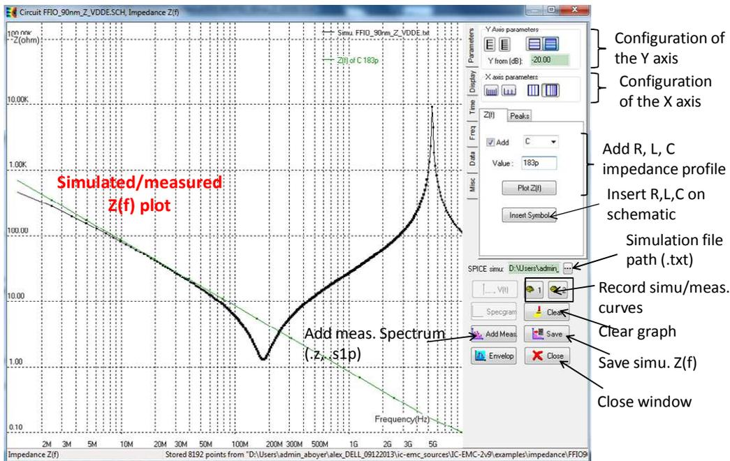
Figure 3- 16: Input impedance simulation performed by WinSPICE (examples/impedance/FFIO90/FFIO\_90nm\_Z\_VDDE.sch)
