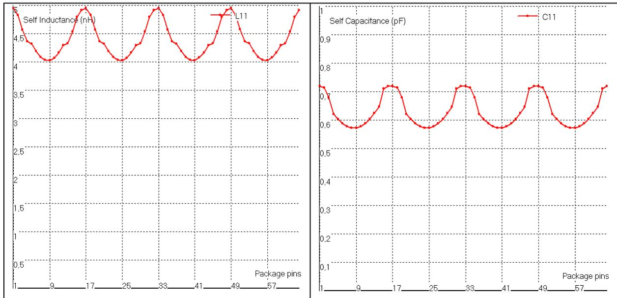
Figure 3- 93 : Simulation of the partial self inductance (on the left) and capacitance (on the right) (examples\package\TQFP64.geo)
