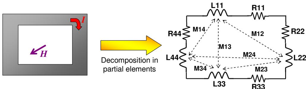
Figure 3- 86 : Decomposition in partial elements of a rectangular loop
