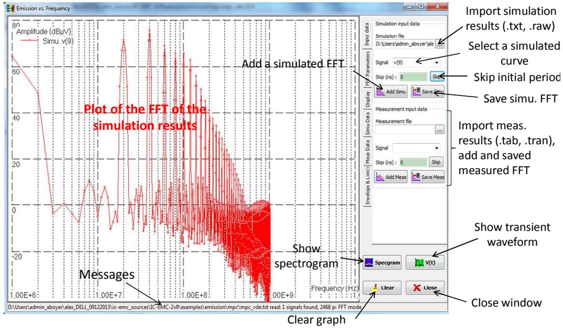
Figure 3- 8: Simulation of the microcontroller's conducted emission (examples\emission\mpc\mpc\_vde.sch)
