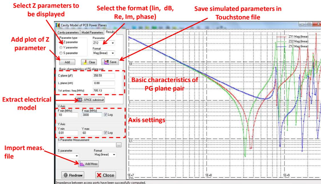
Figure 4- 42: Cavity resonator model: A result plot
