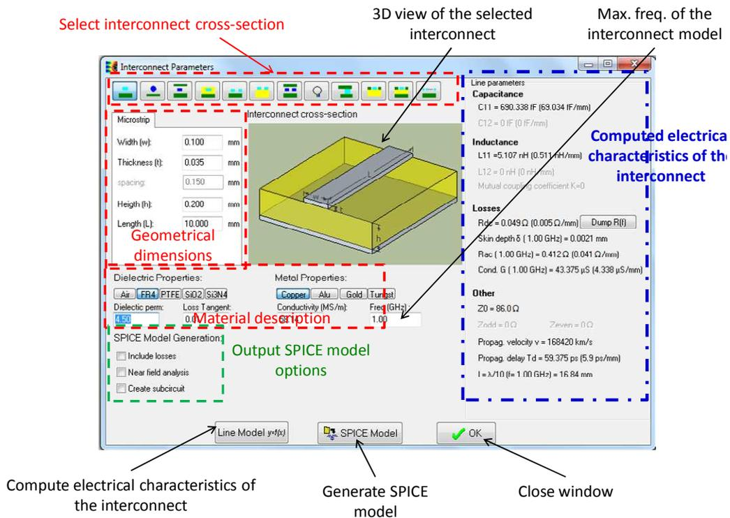
Figure 3- 65: Description of "Tools > Interconnect Parameters"
