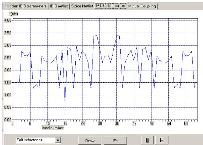
Figure 3- 83: Inductance variation versus lead number (examples\ibis\BGA64.ibs)
