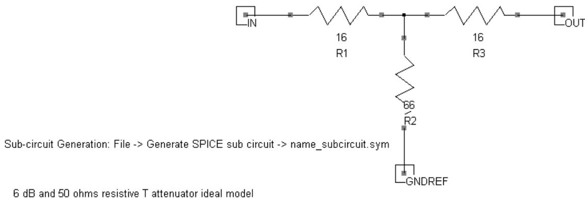
*Figure 4- 8: Placement of subcircuit I/O on a schematic to generate a SPICE subcircuit (examples\EMC\_lib\attenuator\_6dB\_subcircuit.sch)*
