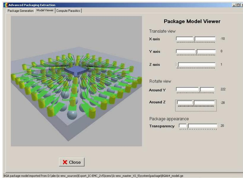
Figure 3- 98 : Constructed model of a BGA 64 (examples\package\ BGA\_model.geo)
