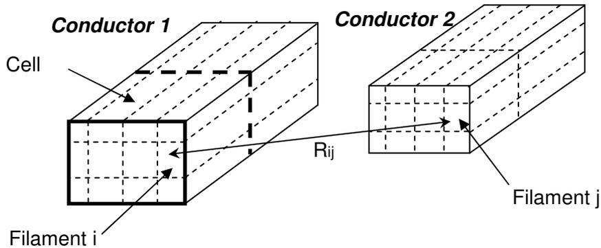
Figure 3- 87 : Meshing in elementary filaments of two conductors
