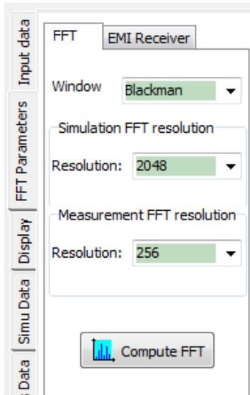
The FFT resolution can be adjusted for the simulation and measurement results independently. The FFT resolution for the measurement results is visible only if a transient measurement results in .tran format has been imported. The number of points which form a displayed FFT result is equal to  $N/2$ . The frequency resolution  $\Delta f$  is given by equation 3-2 and the maximum frequency  $F_{\max}$  by equation 3-3.
