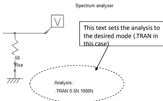
Figure 3- 4: Defining the SPICE simulation parameters
