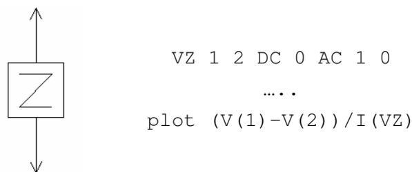
Figure 3- 12: Impedance probe and associated SPICE description
