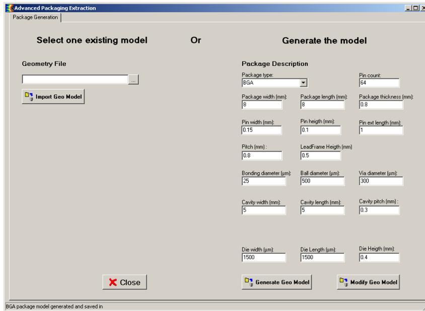
Figure 3- 94 : Launch the BGA model manual construction
