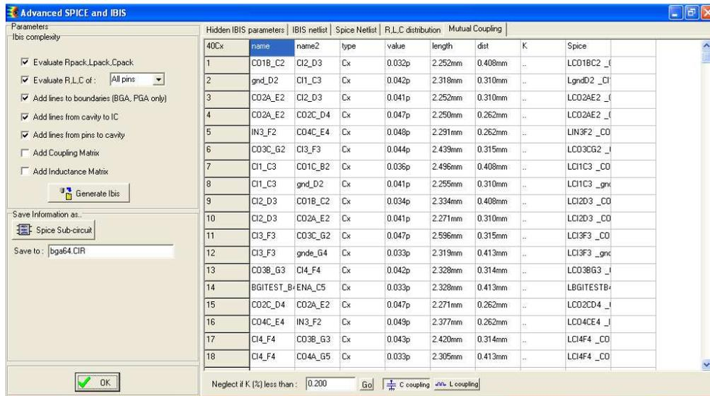
Figure 3- 84: Inductance coupling listed in IC-EMC (examples\ibis\BGA64.ibs)
