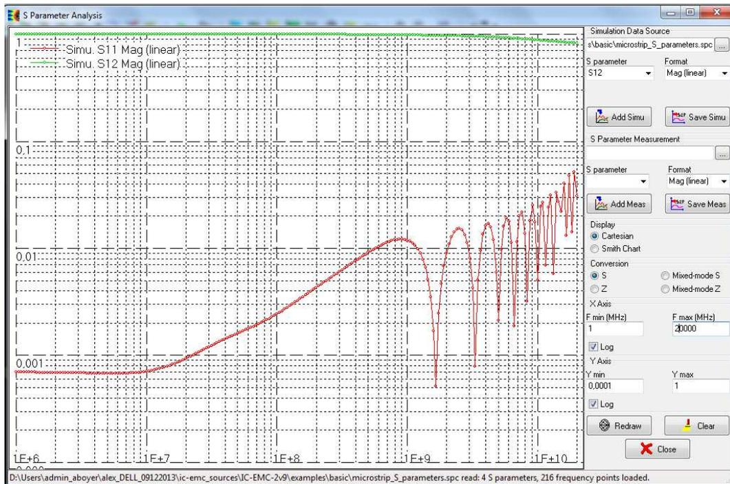
Figure 3- 70: S parameter simulation of microstrip line
