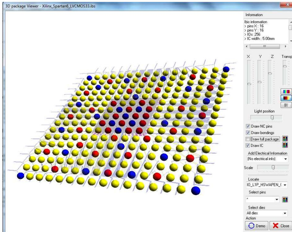
Figure 3- 35 : 3D view of a BGA package (case study/tricore/infineon\_tc1796\_v2.ibs)
