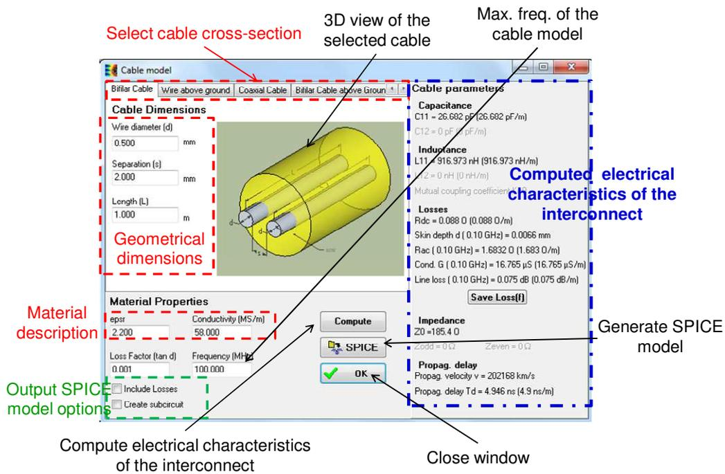
Figure 3- 71: Description of "Tools > Cable Modeling"
