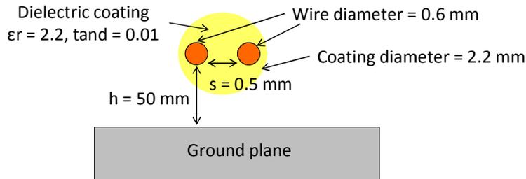
Figure 3- 72: Geometry of the modeled cable
