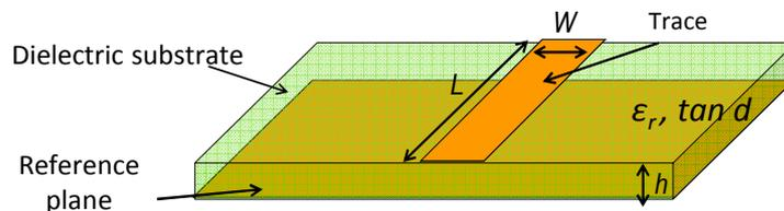
Figure 3- 64: Geometry of the modeled microstrip line
