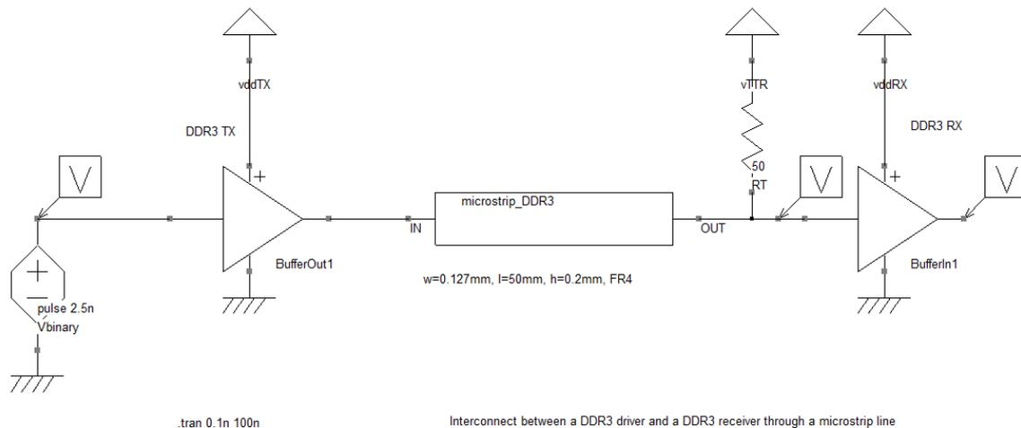
Figure 3- 44: Model of a DDR3 memory link (`\examples\transient\DDR3_link_400MHz.sch`)
