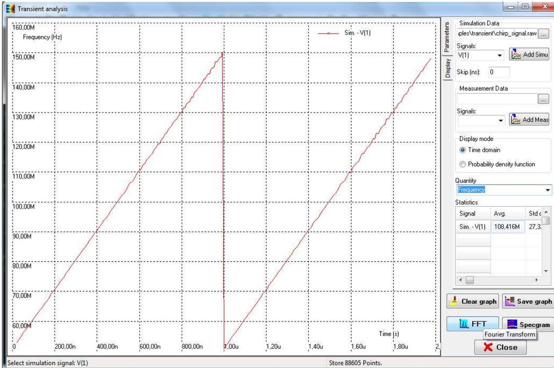
Figure 3- 39 : Evolution of the instantaneous frequency of the simulated chirp signal
