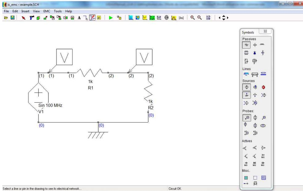
Figure 2- 15: View the nodes of the schematic diagram (icon
