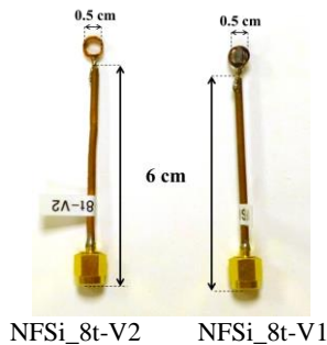
Fig 2. Dimensions of the tested near-field injection probe
