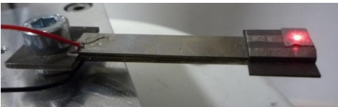
Figure 3. Highly coupled piezoelectric harvester
