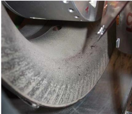
Fig. 20 Wear pattern of the casing
