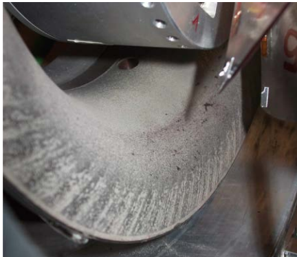
Fig. 20 Wear pattern of the casing
