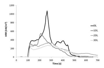
Fig. 6. Heat release rate curves for epoxy cured with amine (D230) and ionic liquid (IL169) in cone calorimeter test (heat flux  $35 \text{ kW/m}^2$ ).
