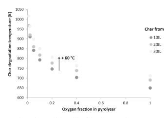
Fig. 11. Thermo-oxidative stability of chars from cone calorimeter tests.
