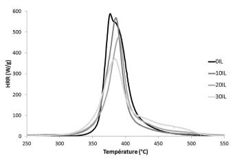
Fig. 4. Heat release rate curves for epoxy resins in PCFC test.
