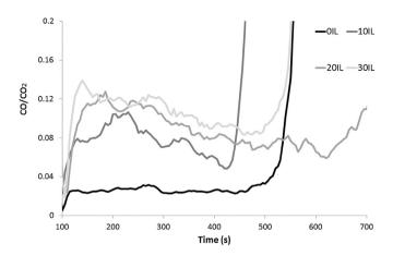
Fig. 8. CO/CO<sub>2</sub> ratio curves for the epoxy resins during cone calorimeter tests.
