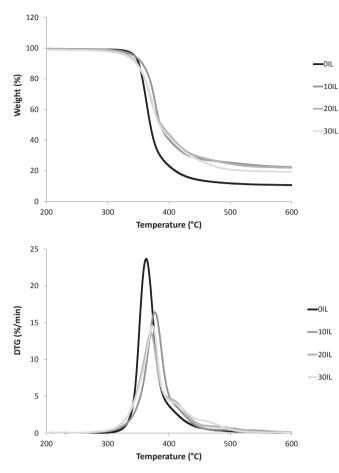
Fig. 3. TG (top) and DTG (bottom) curves for studied epoxy resins (under nitrogen flow).
