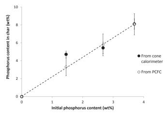
Fig. 10. Phosphorus content in char for residues sampled from cone calorimeter and PCFC tests.
