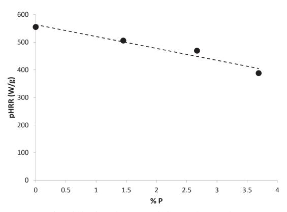
Fig. 5. Peak of heat release rate in PCFC test versus phosphorus content in epoxy networks.
