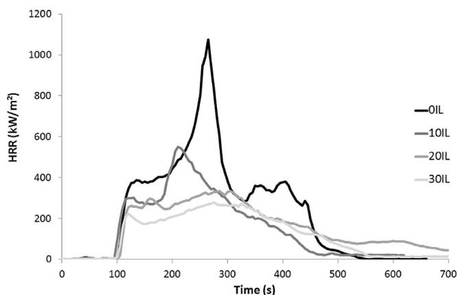
Fig. 6. Heat release rate curves for epoxy cured with amine (D230) and ionic liquid (IL169) in cone calorimeter test (heat flux 35 kW/m<sup>2</sup>).
