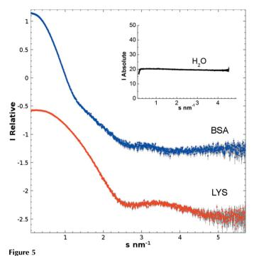
Buffer-subtracted experimental scattering pattern from bovine serum albumin (BSA) and lysozyme (LYS) scaled for visualization. The inset graph represents scattering from water (with empty capillary background subtracted), which was used for the absolute intensity calibration of sample curves.
