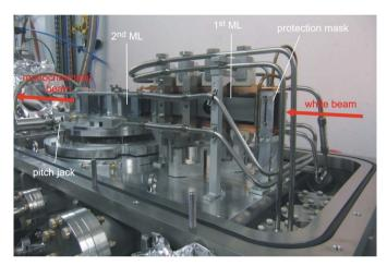
Figure 2 Inside view of the double ML monochromator vessel.
