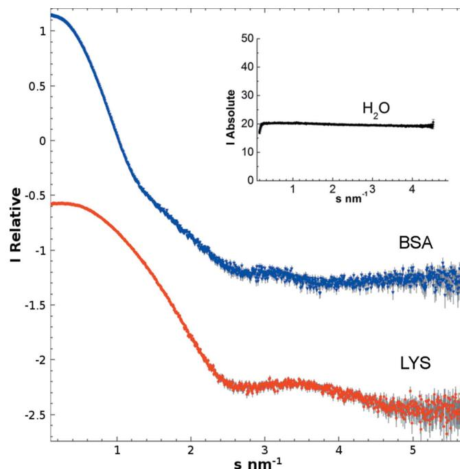
**Figure 5** Buffer-subtracted experimental scattering pattern from bovine serum albumin (BSA) and lysozyme (LYS) scaled for visualization. The inset graph represents scattering from water (with empty capillary background subtracted), which was used for the absolute intensity calibration of sample curves.
