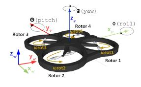
Fig. 3. Quadrotor system.
